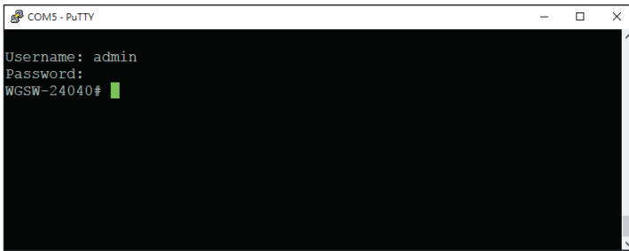
Figure 3-3: Managed Switch Console Login Screen
